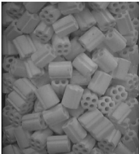
FIG. 21. Randomly packed tube packed with reforming catalyst.
